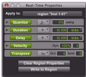
Real-Time Properties window with properties enabled
