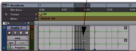
Applying Range Warp to a selection between bounding Warp markers
