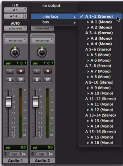
Output Path selector, Mix window
