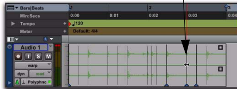
Applying Range Warp between two Warp markers in a region
