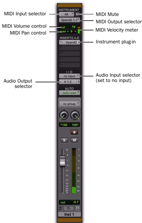
Instrument track configured to control and monitor an instrument plug-in (Digidesign Xpand 2 )
