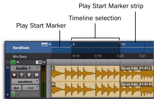
Dynamic Transport mode, Play Start Marker shown in expanded Main Timebase ruler
