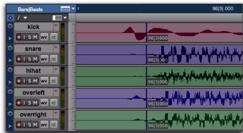
Figure 31. Overhead mics generate late beat triggers
