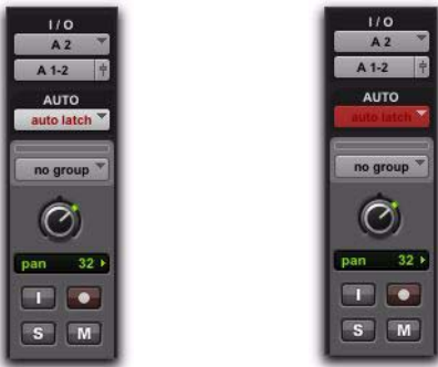
Automation Mode selector showing enabled state (left) and writing state (right)
